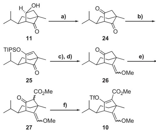
**Scheme 3.** Reagents and conditions: (a) Jones reagent, acetone, rt, 15 min, 95%. (b) TIPS-Cl, NaHMDS, THF,  $-78$  °C, 1.5 h, 98%. (c)  $\text{Ph}_3\text{PCH}_2(\text{OMe})\text{Cl}$ , *n*-BuLi, THF, 60 °C, 4 h. (d) TBAF, THF, 0 °C, 1 h, 73% in two steps. (e) NaHMDS,  $\text{CNCO}_2\text{Me}$ , THF,  $-78$  °C, 30 min, 87%. (f) NaHMDS,  $\text{TiO}_2$ ,  $\text{Et}_2\text{O}$ ,  $-78$  °C, 1.5 h, 94%.
