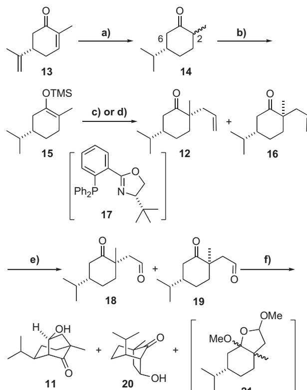
**Scheme 2.** Reagents and conditions: (a) H<sub>2</sub> (4 MPa), Rh/Al<sub>2</sub>O<sub>3</sub> (0.1 mol %), EtOH, rt, 3.5 h, 96%. (b) TMSCl, NaI, Et<sub>3</sub>N, MeCN, rt, 4 h, 99%. (c) MeLi, DME, -40 °C then allyliodide, THF, -50 °C, 22 h, 97% (12/16=3.4:1). (d) TBAT, Pd<sub>2</sub>(dba)<sub>3</sub>, 17, THF, allyl carbonate, 78%, (12/16=55:1). (e) O<sub>3</sub>, CH<sub>2</sub>Cl<sub>2</sub>, then Et<sub>3</sub>N, -78 °C, 3 h, quant. (f) KOH, EtOH, 50 °C, 13 h, 80%, recrystallization.
