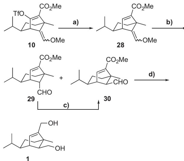
**Scheme 4.** Reagents and conditions: (a)  $\text{Pd}(\text{OAc})_2$ ,  $\text{HCO}_2\text{H}$ ,  $\text{PPh}_3$ , *n*-Bu<sub>3</sub>N, DMF, 50 °C, 0.5 h, 96%. (b)  $\text{HClO}_4$ ,  $\text{Et}_2\text{O}$ , rt, 97% (**29/30**=1:2.5). (c) Morpholine, PTSA, MeCN, rt, 14.5 h, 94% (**29/30**=1:2.3). (d) DIBAL,  $\text{CH}_2\text{Cl}_2$ ,  $-78$  °C, 1 h, 89%.
