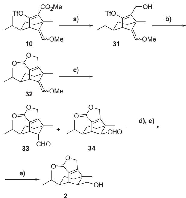
**Scheme 5.** Reagents and conditions: (a) DIBAL, CH<sub>2</sub>Cl<sub>2</sub>, –78 °C, 45 min, 95%. (b) Pd(PPh<sub>3</sub>)<sub>4</sub>, CO atmosphere, LiCl, *n*-Bu<sub>3</sub>N, MeCN, 60 °C, 4 h, 88%. (c) HClO<sub>4</sub>, Et<sub>2</sub>O, rt, 2 h, 91% (**33/34**=14:1). (d) K<sub>2</sub>CO<sub>3</sub>, MeOH, rt, 3 h, 70% (**33/34**=1:2.6). (e) NaBH<sub>4</sub>, MeOH, 0 °C, 2 h, 44%.
